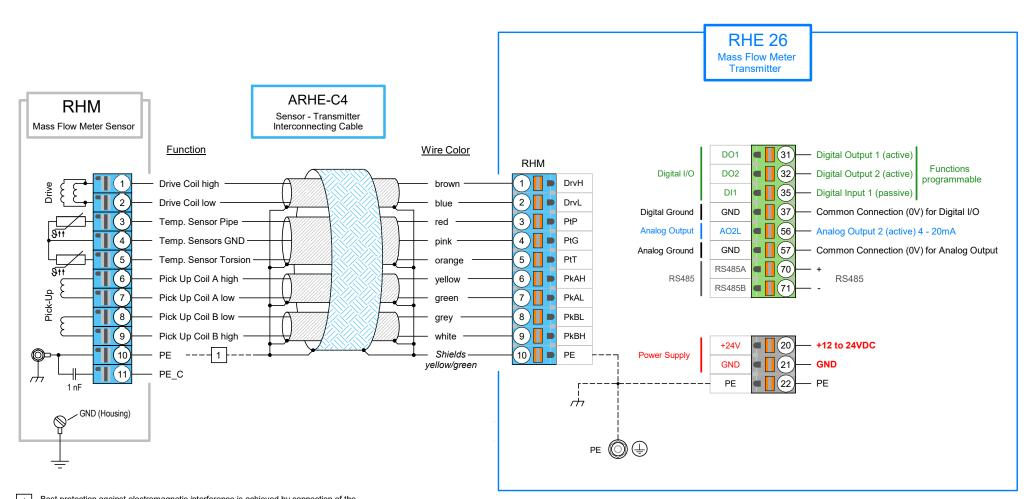
Best protection against electromagnetic interference is achieved by connection of the cable screens to PE.
